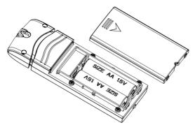
Figure 3: Sensor battery installation
