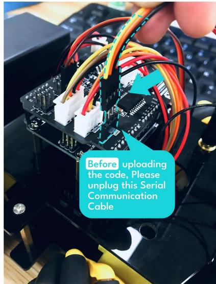
⑫ Upload the program to the ESP32-CAM control board.
