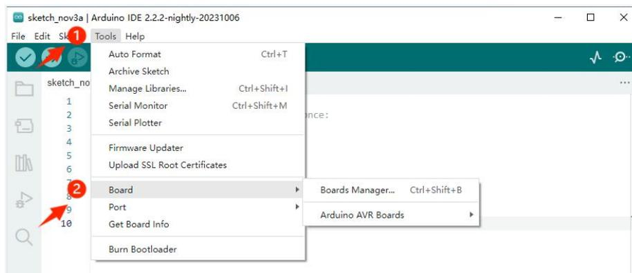
This time we use the control board is the ESP32 control board, so we need to install the ESP32 board in the Arduino IDE. Follow these steps:
