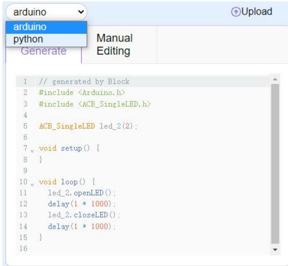
3. Click the "Upload" button to upload the program. When the upload progress reaches 100%, it is successful. After the upload is successful, the program can be run on the ESP32 controller board without the computer, that is, you can unplug the data cable and let the program run independently on the ESP32 (connect the ESP32 to an external power supply).
