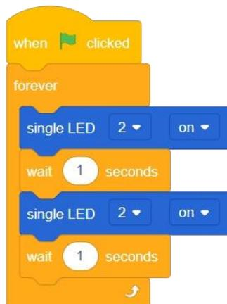
2. After writing, debug the code online. Click the code to run it. The code will turn yellow, indicating that the code is running. The LED on the ESP32 will repeatedly light up for 1 second and then go off for 1 second. Click on the code again to stop running it.
