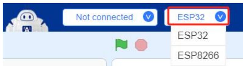
2.Find the serial communication connection button in the ACECode interface.
