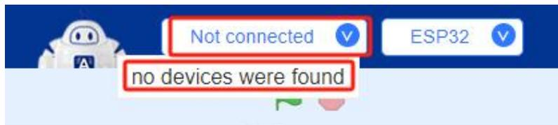
3. When we connect ESP32 to the computer with a data cable, a new port will be added to the serial communication port information list. The port number is random and will change according to the actual situation. Click the newly added port to establish a communication connection between ACECode and ESP32. After the connection is successful, the connection status display on the connection button will switch from "Not connected" to the information of the connected port.
