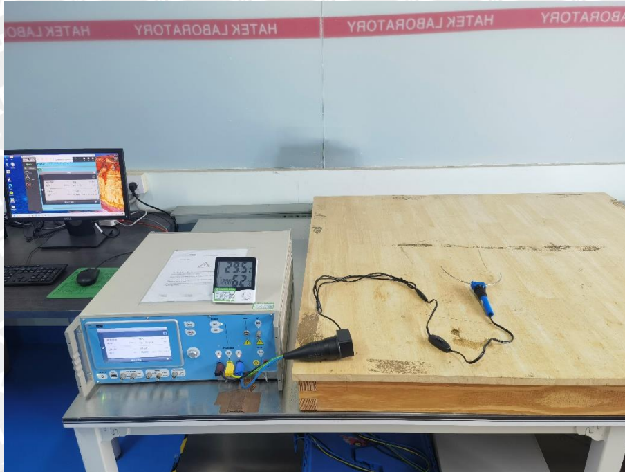
Photograph 3: Set-up for EFT, Surge and Voltage Dips
