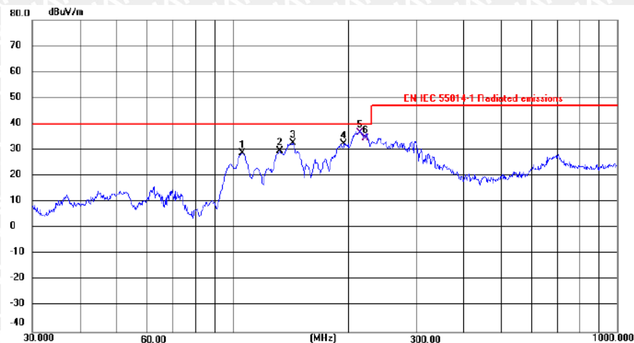
Figure 5: Test Curve of Radiated Emission in the frequency range of 30-1000MHz, Horizontal (AC 230V)
