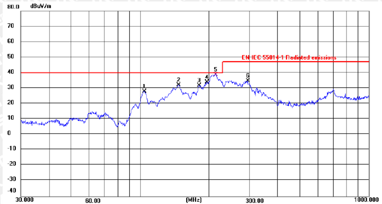
Figure 3: Test Curve of Radiated Emission in the frequency range of 30-1000MHz, Horizontal (AC 120V)
