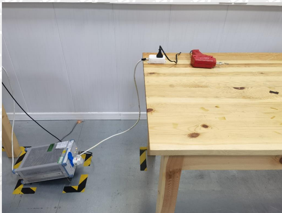
Photograph 1: Set-up for Disturbance Voltage
