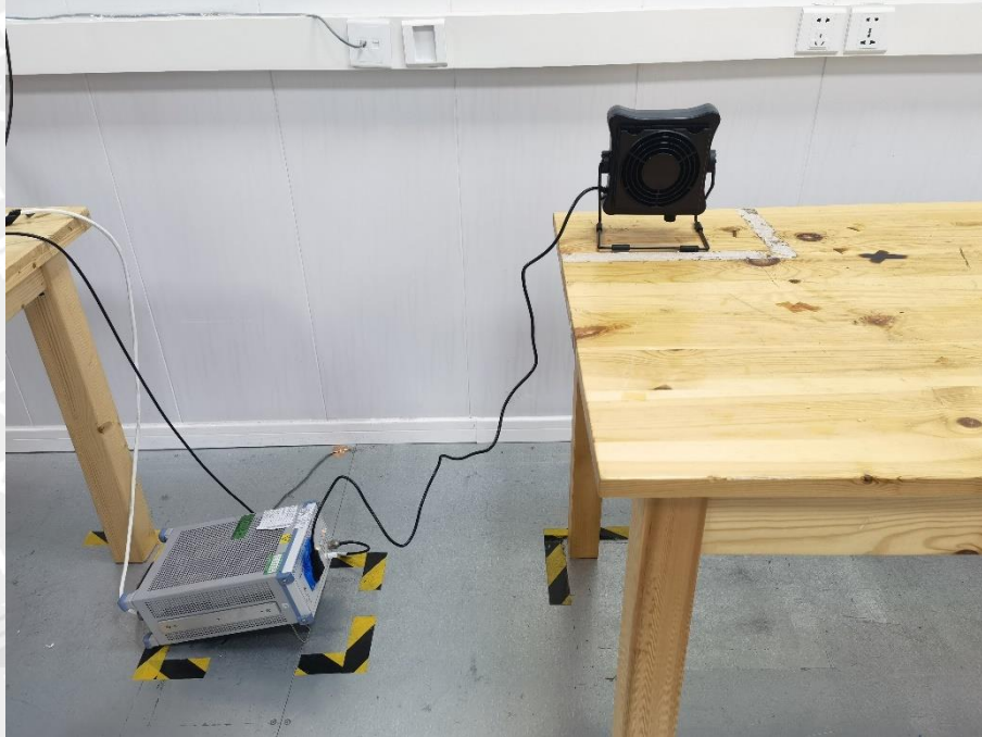
Photograph 1: Set-up for Disturbance Voltage
