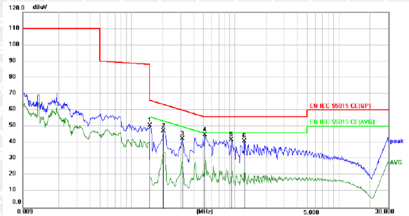
Figure 2: Spectral Diagrams, Conducted Emission, 0.009-30MHz, N
