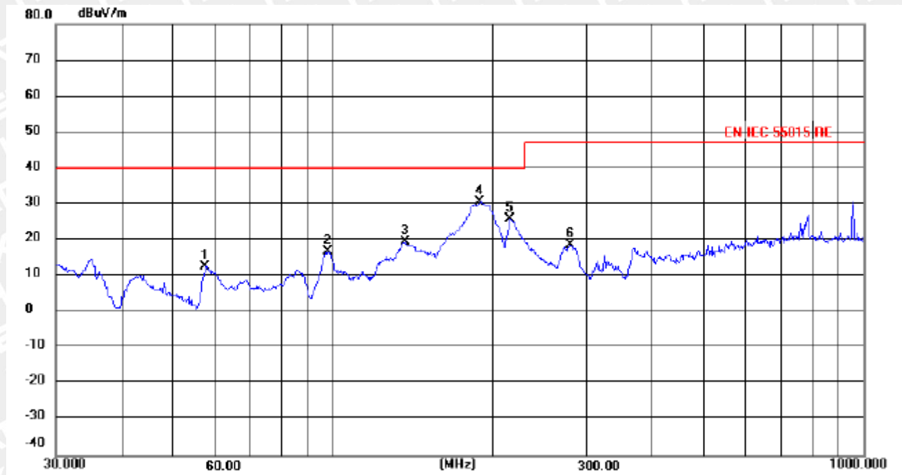
Figure 6: Spectral Diagrams, Radiated Emission, 30MHz-1000MHz, Horizontal
