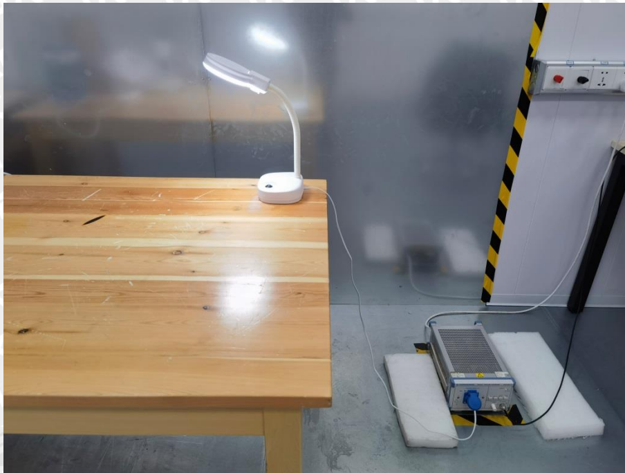
Photograph 1: Set-up for Disturbance Voltage
