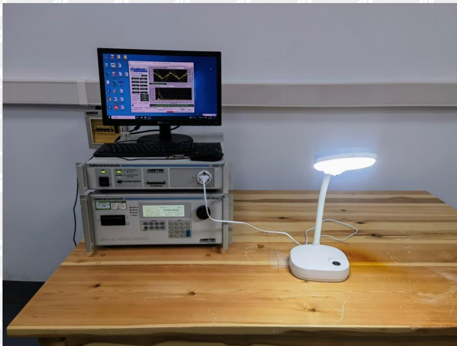
Photograph 2: Set-up for Harmonics, Voltage Fluctuation and Flicker
