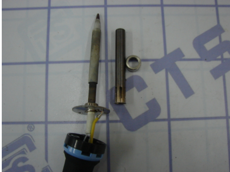
Figure 9 (Internal view of iron)
