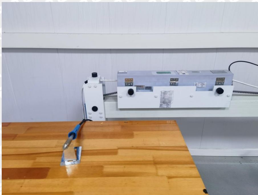
Photograph 2: Set-up for Disturbance Power
