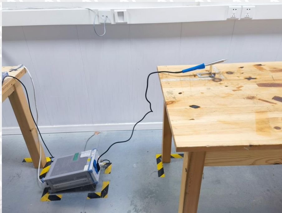
Photograph 1: Set-up for Disturbance Voltage
