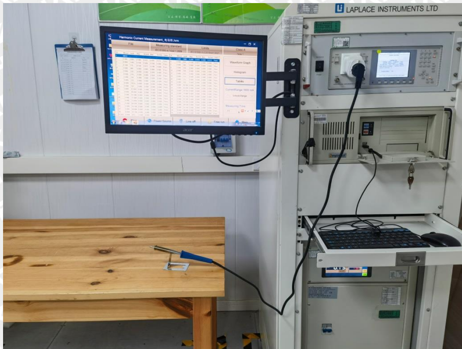
Photograph 3: Set-up for Harmonics, Voltage Fluctuation and Flicker
