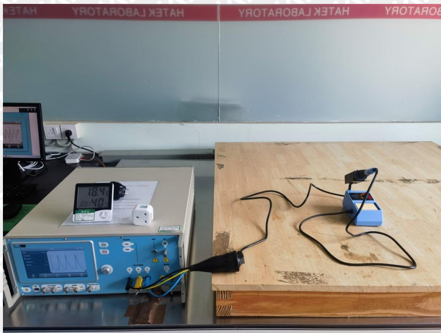
Photograph 3: Set-up for EFT, Surge and Voltage Dips
