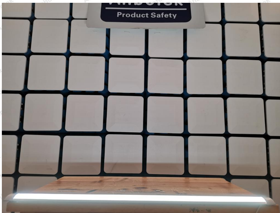
Photo of RF Field Strength susceptibility Test
