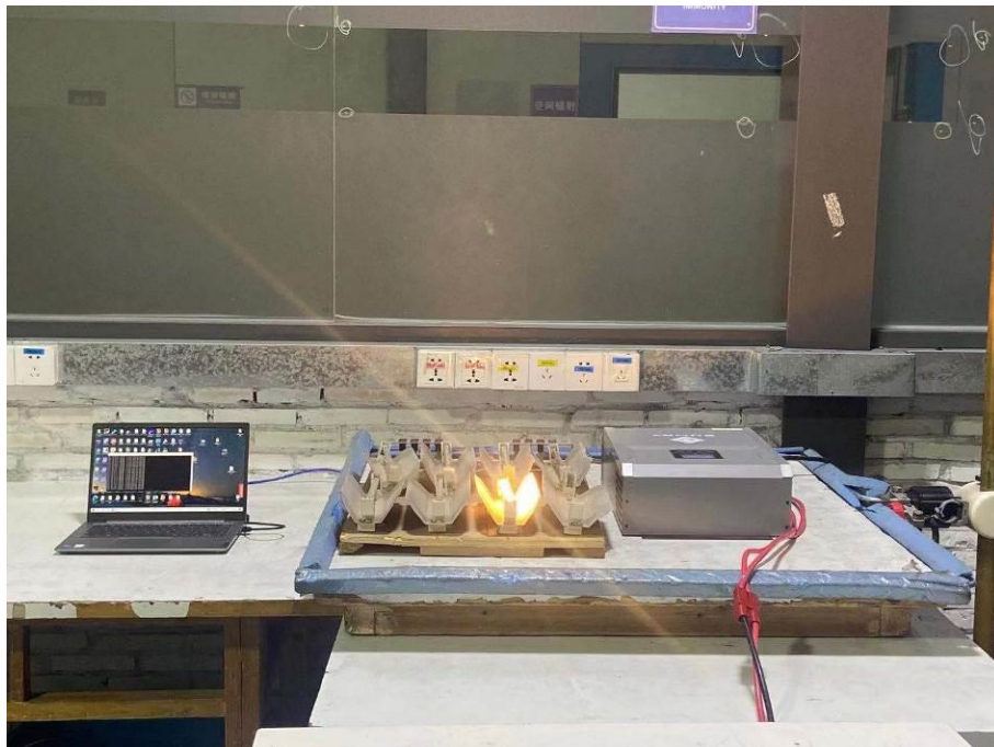
16.10.Photo of Magnetic Field Immunity Test
